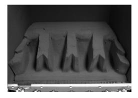
b) Position the two halves of the front ceramic (L/H & R/H) on the locating channel in the front ceramic, ensuring it is located onto the lip on the burner front ceramic support. (See fig. 2 below)
